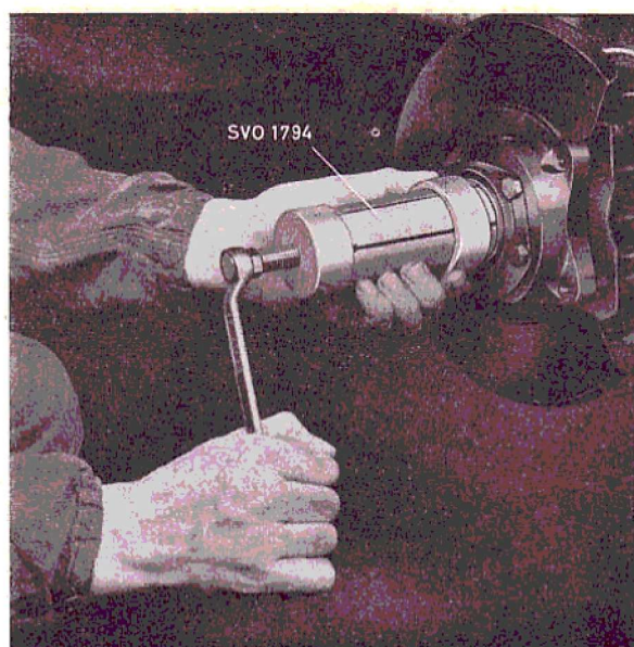
Fig. 18. Removing the inner bearing.
